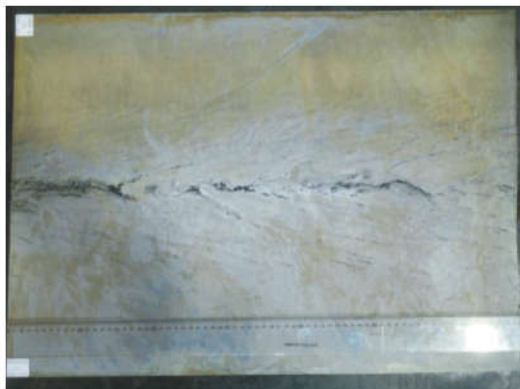
图 3 H13 钢 \Phi 380 mm 连铸圆坯纵剖酸洗宏观组织形貌 Fig. 3 Macrostructure morphology of longitudinal section pickling H13 steel \Phi 380 mm continuous casting round bloom
